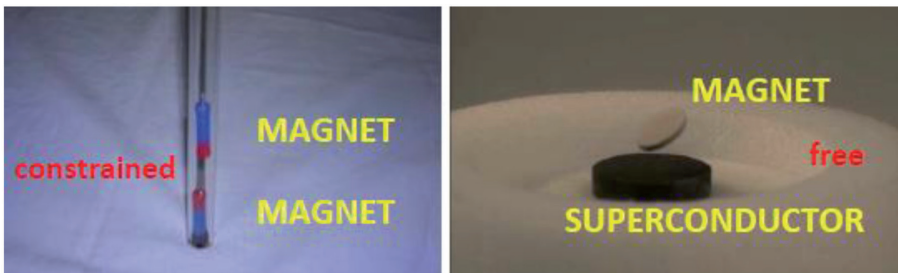
Fig. 12. The phenomenology of a free magnet repelled by a YBCO tablet is not amenable to the situation in which two constrained magnets interacts repelling each other.
