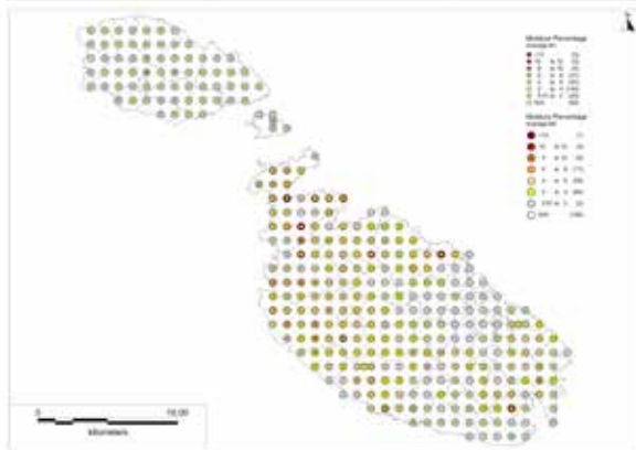
Figure 5a: Average moisture content values for M1 (2003) as the smaller circles and M2 (2013) values as the larger circles surrounding the smaller (M1) circles
