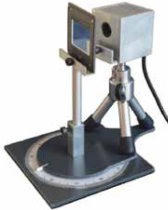
Figure 9. SPETTROGRAFO system used as an optical goniometer.
