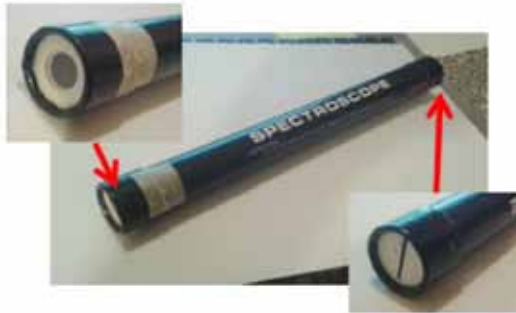
Figure 2. A simple spectroscope: the grating and slit are evidenced.
