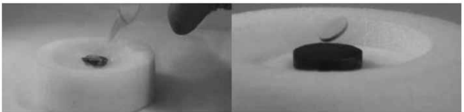
Fig. 11. A cooled tablet of YBCO interacts in a new way with a magnet. How can be this behavior interpreted?
