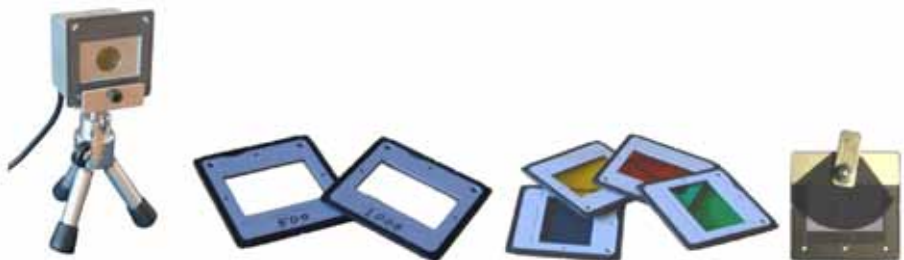
Figure 4. SPETTROGRAFO system (left) and accessories: diffraction gratings, coloured and Polaroid filters (right).
