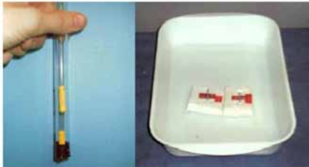
Fig. 1. Magnets do not attract or repel each other according to the poles: this is true only if they are constrained. If the magnets are free, only attraction or rotation followed by attraction occur.
