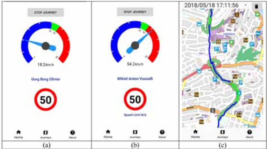
Fig.4. The mobile app display, (a) Home interface, (b) Notification shown when speed limit defaults to 50km/hr , (c) Saved journey viewer
