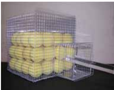
Figure 1 - The model: the box with pistons and the transmission of pressure
