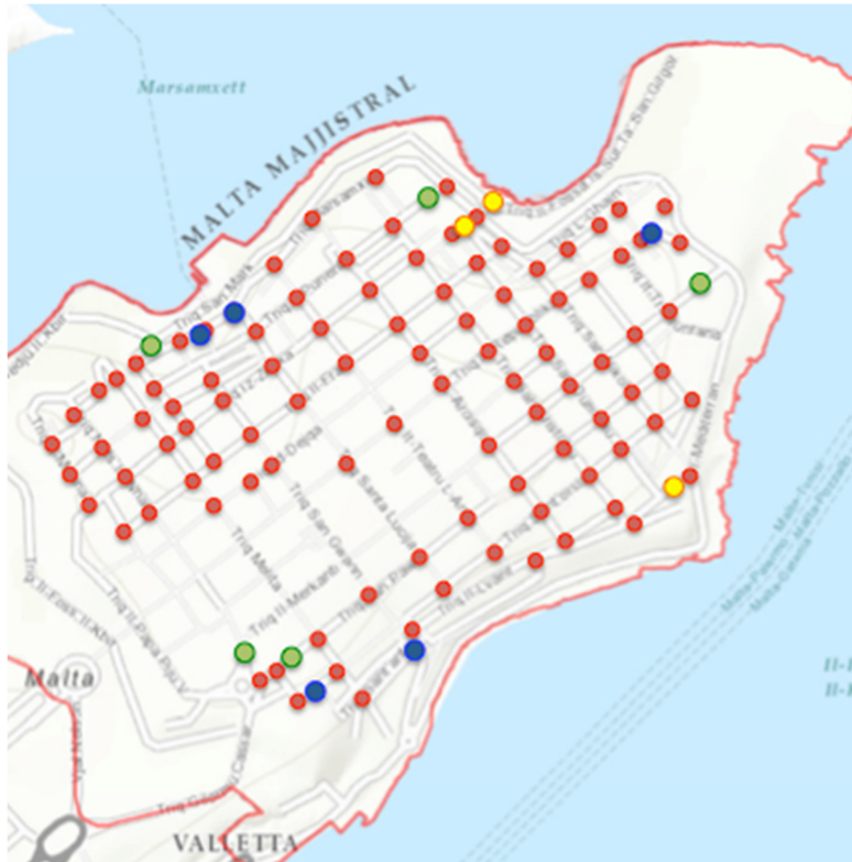
Fig. 1: Map of Valletta showing the entry and exit points of the city. The green dots represent the entry points; the blue dots represent the exit points whilst the yellow dots represent two-way roads (entry and exit). The red dots represent the location of around 80 beacons practically in each and every junction in the city (drawn up by author using https://www.openstreetmap.org ).
