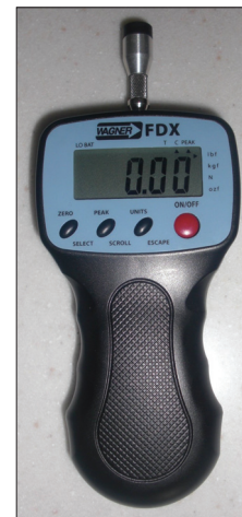
Figure 3: PainTest™ FPX 25 Algometer (Wagner Instruments, Greenwich, USA)
