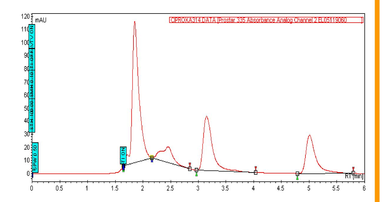
Figure 1: Chromatogram of Ciprofloxacin 2.5μg/ml (retention time: 3.15 minutes) with Sulfadimidine (retention time: 5.01 minutes)
