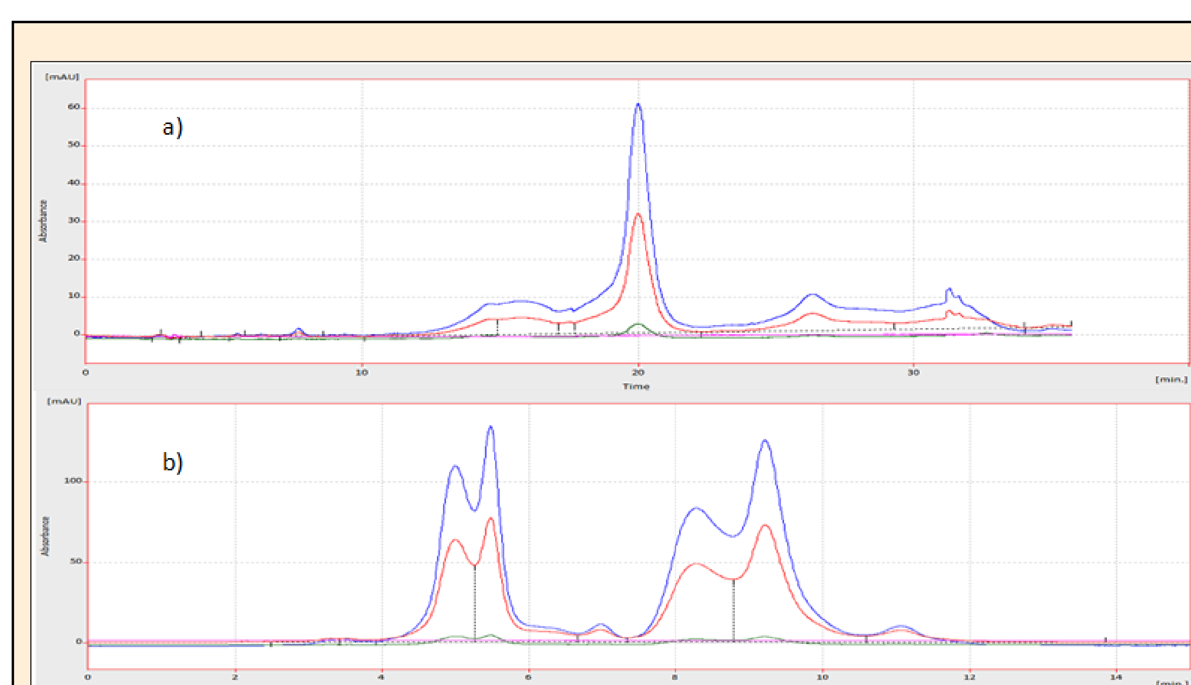
Figure 2: Separation at different wavelengths (220nm, 240nm, 280nm, 600nm) using the mobile phase composition a) methanol/water (6:4) b) acetonitrile/water (6:4)
