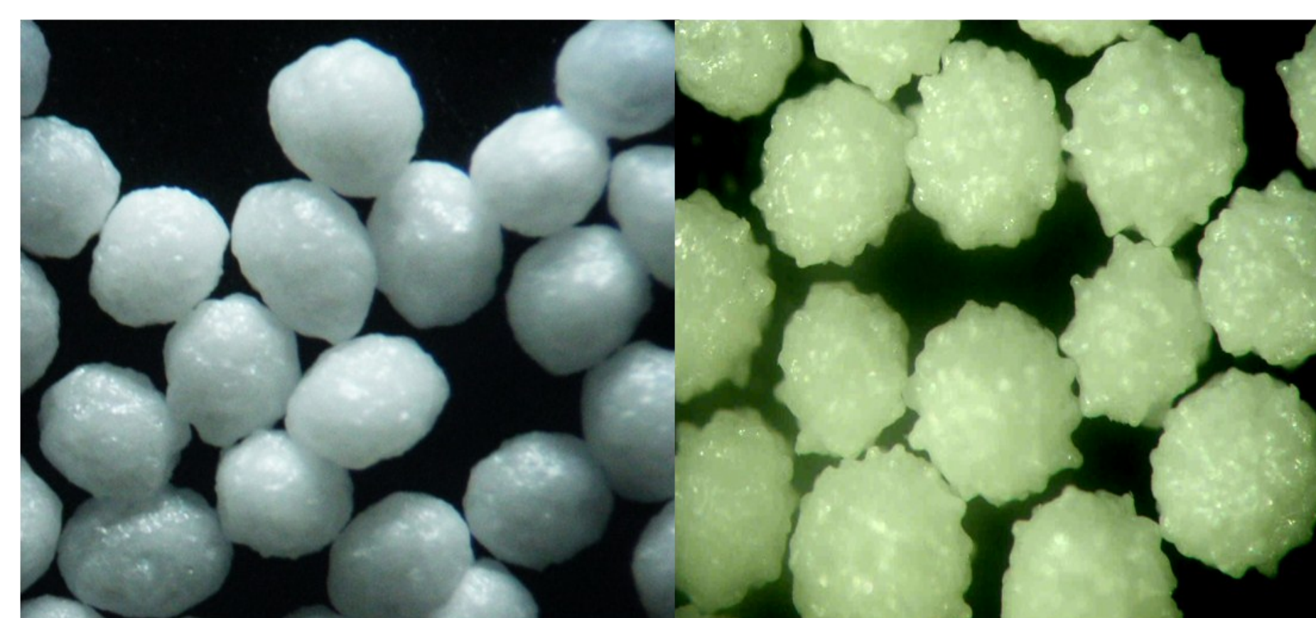
Figure 1. Pellets as seen under a microscope (Left — pellets with a very smooth surface, rated 5; Right — pellets with a rough surface, packed with large spikes, rated 1).
