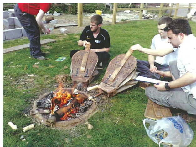
Figure 1. Testing temperatures and recording data during a copper smelting experiment (photograph by C. Busuttil 2011).
