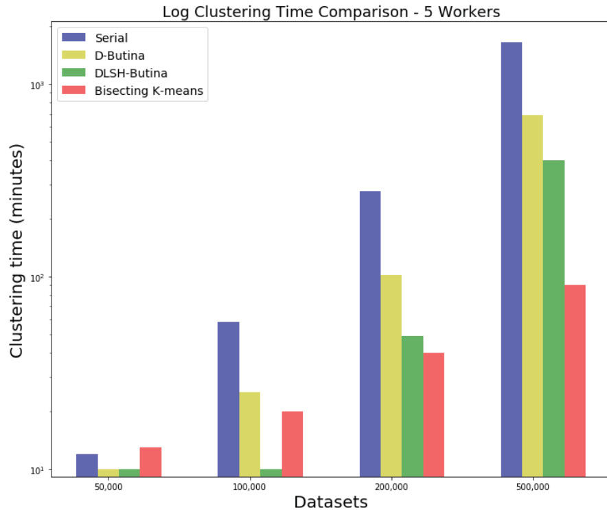
Figure 4.3: Comparison of the speed performance in logarithmic scale of the algorithms on the four datasets when using 5 worker nodes.
