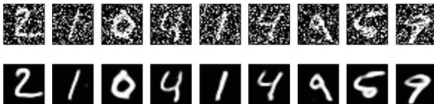
Figure 2.11: Denoising AutoEncoder. Top: Noisy images fed to the model, Bottom: Reconstructed by the model Source: Chollet [15]
