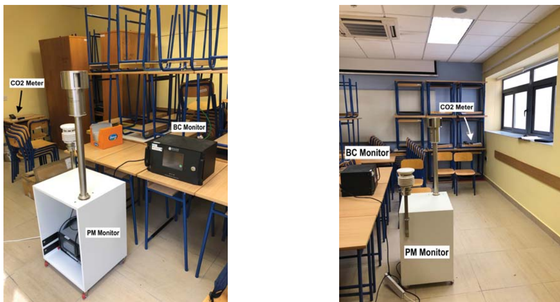
Figure 2.4: Indoor equipment including the PM and BC monitors as well as CO 2 meters.
