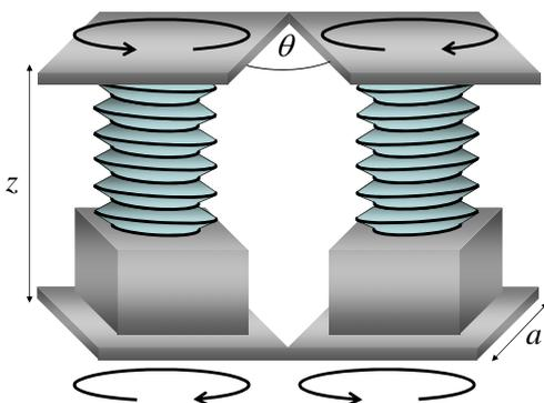
Also, provided that the pitch of the tread is sufficiently large, when loaded in the third direction the "bolt" and the "nut" will slide past each other causing a decrease in the third dimension together with a rotation of the "bolt" and the "nut". This will cause the squares connected to them to rotate, that under the right conditions, will induce a decrease in size in the orthogonal directions.
