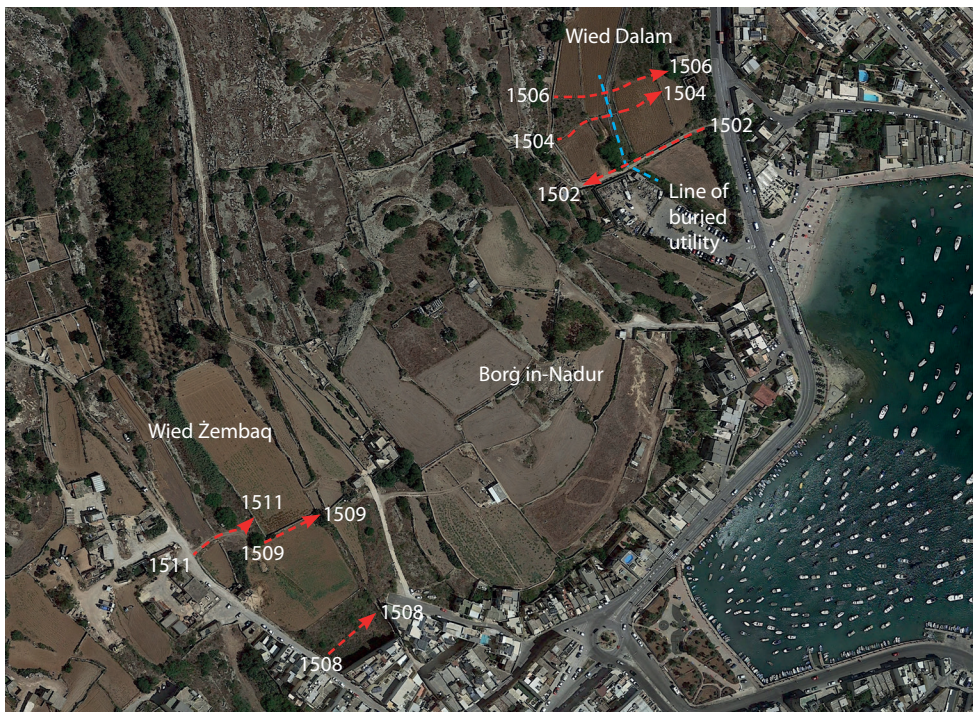
Figure 2.3. The location of the Birżebbuġa Wied Dalam and Wied Żembaq basins and their GNSS-located GPR lines (A. Ruffell; image © 2020 Google).
