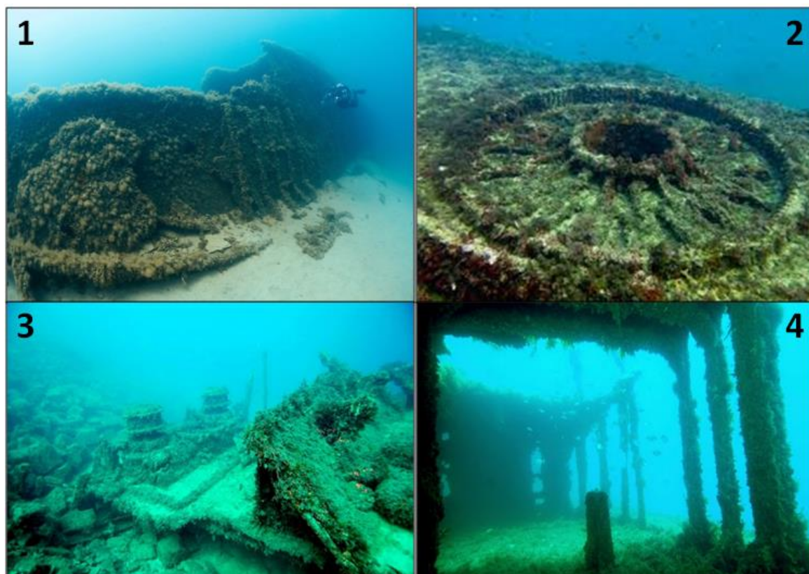
Figure 9. Diver passing along the starboard side (1), mounting base for twin 4.7in gun (turret) (2), forepart (forecastle deck) leaning on the rocky slope - breakwater and anchor windlass can be seen (3), a section of the upper structure before 2019 with shoals of fishes (4) (Source: Google)
