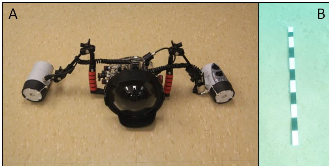
Figure 11. Underwater camera housing (Ikelite) used for 3D survey, with two strobe lights and a hemispherical dome port (A), Scale bar used for the survey (B) (Source: K. Yamafune)
