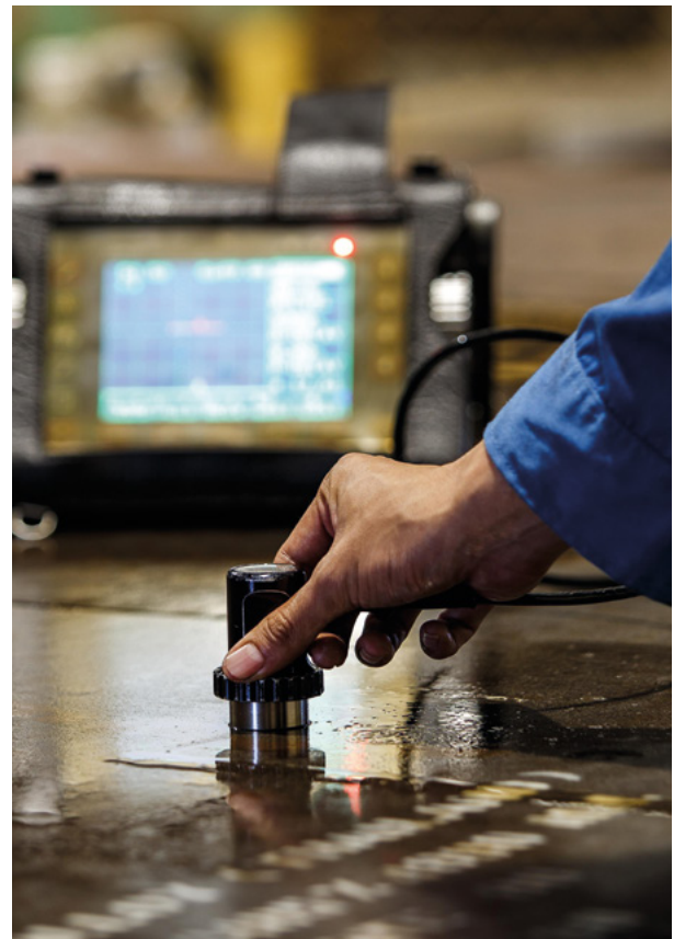
Top: Maria in Chinatown in central Singapore. Bottom left: Maria in Little India in Singapore. Bottom Right: Steel plate being inspected for internal defects using ultrasonic testing. Opposite Page: Maria descending from the summit of Mount Rinjani in Indonesia.
