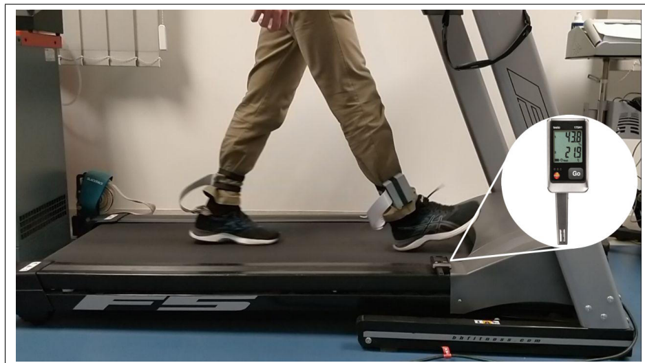
Figure 4.13: The setup used for the walk trials - subject wearing the system prototype and walking on a treadmill, with the Testo logger monitoring the ambient temperature.
