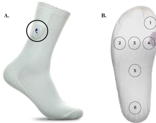
Figure 2.18: Siren Diabetic Socks: (a) image of socks showing (circled) processing unit location; (b) image of the bottom of the sock showing sensor locations (adapted from [22]).
