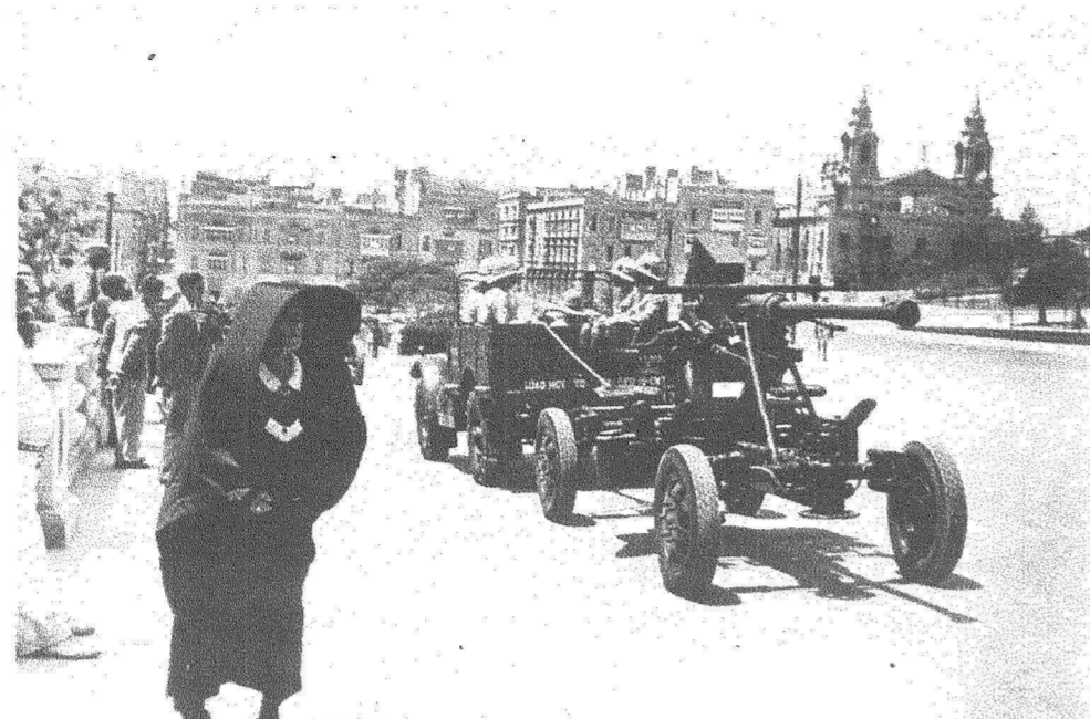
A military vehicle pulling a 40mm Bofors Light Anti-Aircraft Gun down Giloramo Cassar Avenue, Valletta.
