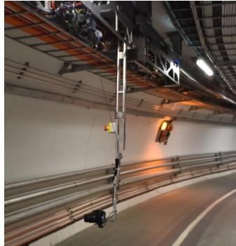
Figure 4.2: Camera on the arm extending from one of the wagons of the TIM
