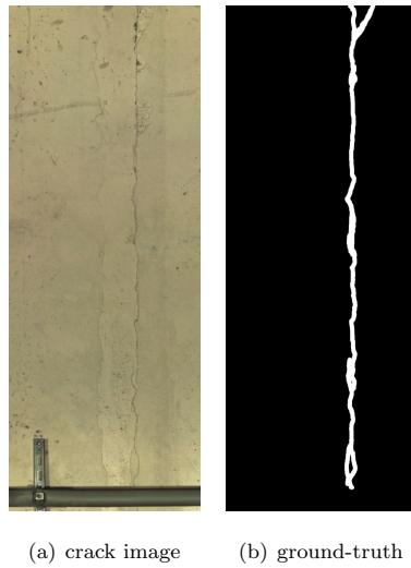
Figure 5: A sample of crack markings from the LHC dataset
