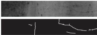
**Fig. 6.** Original image and crack segmentation result from Shen et al. (2015). Reprinted from International Journal of Distributed Sensor Networks, vol. 11, No. 6, B. Shen, W. Zhang, D. Qi, X. Wu, Wireless Multimedia Sensor Network Based Subway Tunnel Crack Detection Method, © (2015) This is an open access article distributed under the Creative Commons Attribution License.
