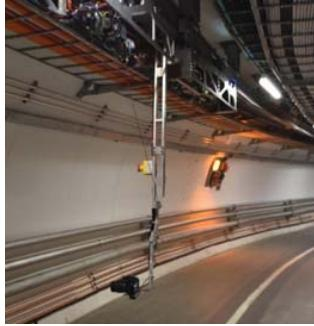
Fig. 1. Camera on the arm extending from one of the wagons of the TIM
