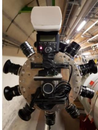
Figure 4.7: Camera rig in the provisional commercial camera system
