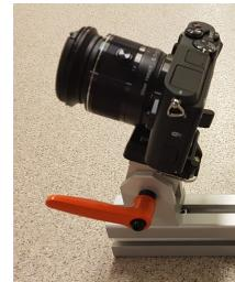
Figure 4.5: Camera attached to a quick release plate
