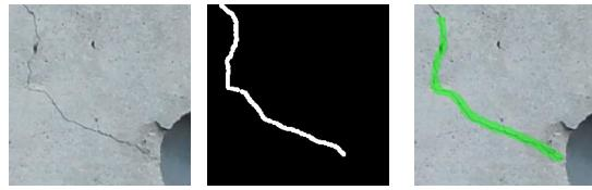
(a) original      (b) ground-truth      (c) Mask R-CNN
