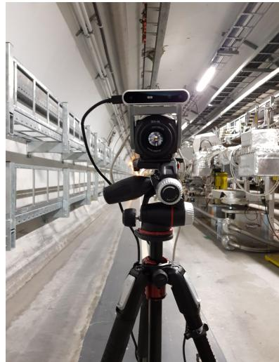
Figure 8.3: Thermal and RGB camera placed on a tripod
