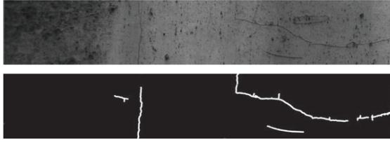
Figure 2.3: Wall image and the result of crack segmentation from [13]
