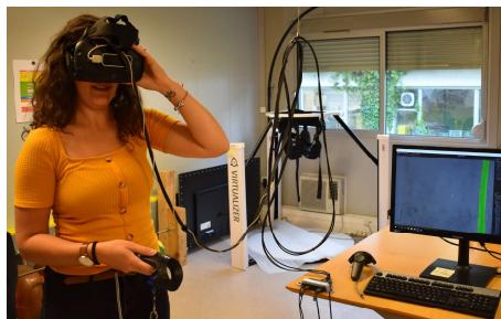
**Figure 7.** Viewing the detected cracks and joints overlayed on the 3D model in VR-SHM
