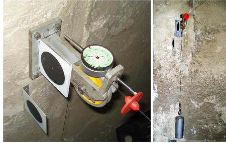
Figure 2.1: Invar wire and gauge used during manual surveys [11]
