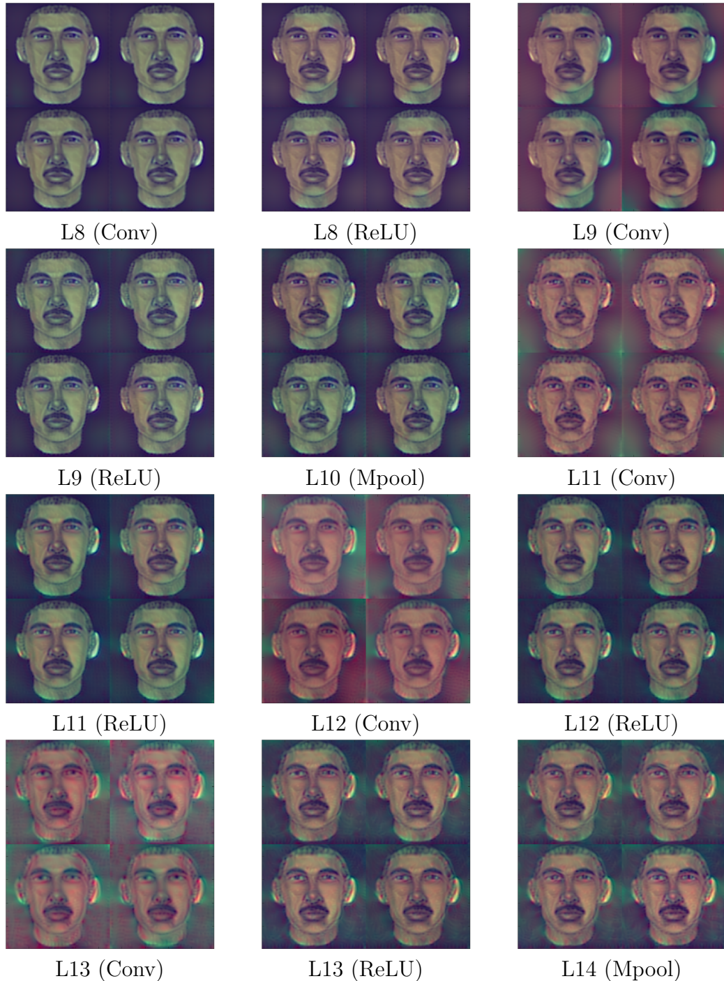
Figure A.14: Visualisation of network (shown in Table 3.1) when using photo/hand-drawn sketch pairs for training and a sketch as input.
