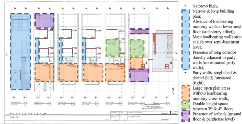
Figure 3-41 Development Permit Drawing of Xemxija Building Number 0011 including the identification of building characteristics, which could influence its structural response (Malta Environment and Planning Authority Mapserver https://www.mepa.org.mt/mepa-mapserver ).
