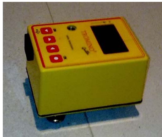
Figure 3-42 A Tromino™ tromograph used for the ambient noise recordings carried out in Xemxija Building Number 0011 by the Seismic Monitoring and Research Unit (SMRU) of the University of Malta.
