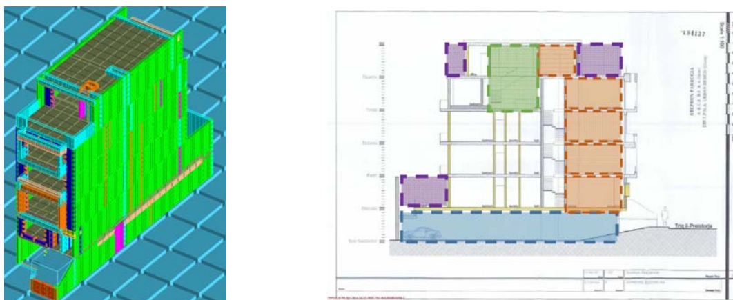
Figure 3-40 Xemxija Building Number 0011: 3-dimensional view of ELS® numerical model and longitudinal section.
