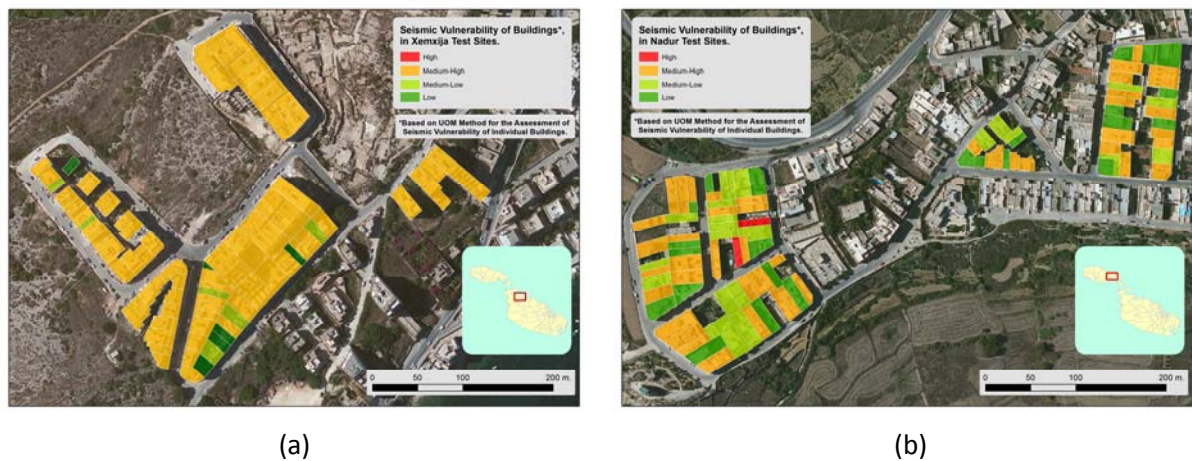
Figure 7: GIS thematic maps indicating the seismic vulnerability rating of the buildings in (a) Xemxija and (b) Nadur Test sites.
