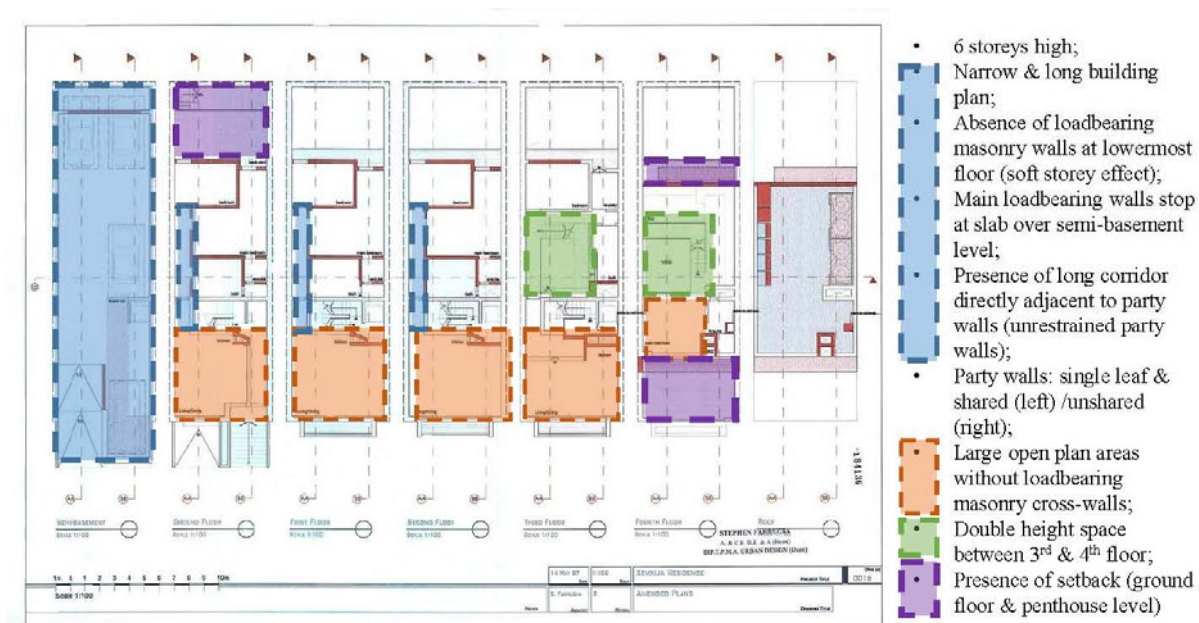
Figure 3: Examples of seismic vulnerability characteristics identifiable on plan in the contemporary loadbearing building typology present in the Maltese Islands (Malta Environment and Planning Authority Mapserver https://www.mepa.org.mt/mepa-mapserver ).
