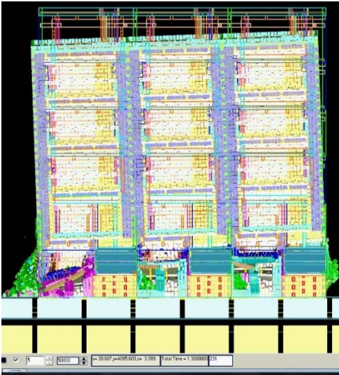
Figure 4-28 Front and isometric view of three-building control model (Model 138) at frame 231 (dynamic loading stage).
