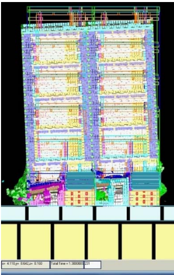
Figure 4-22 Front and isometric view of two-building control model (Model 130) at frame 231 (dynamic loading stage).
