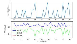
FIG. 9. Validation right after short training of 35 episodes on June 8, 2020. Despite the short training, the agent corrects the trajectory to better than the 2 mm RMS target within 1-3 iterations.
