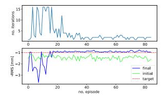
FIG. 13. Online training of NAF agent on LINAC4 trajectory steering in horizontal plane. The maximum allowable RMS was limited to 3 mm due to machine protection reasons. The target for the training was set to reach 1 mm RMS.
