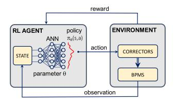
FIG. 2. The RL paradigm as applied to particle accelerator control, showing the example of trajectory correction.
