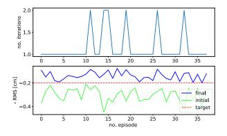
FIG. 10. Validation on accelerator on September 22, 2020, of agent that was trained more than three months earlier (June 10, 2020). The agent corrects the trajectory to better than 2 mm RMS within 1-2 iterations. No retraining was required.
