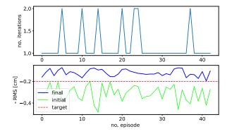
FIG. 11. Validation on accelerator of agent that was trained on simulation. The agent corrects the trajectory to better than 2 mm RMS within 1-2 iterations.
