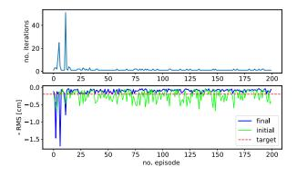
FIG. 6. Online training of NAF agent of AWAKE electron line trajectory steering in the horizontal plane. In the upper plot the number of iterations per episode is given. The lower plot shows the initial and final negative RMS value for each episode. The target negative RMS value is indicated in red.
