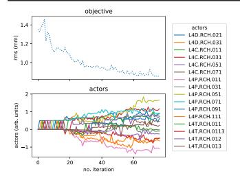
FIG. 12. Optimization with COBYLA of the LINAC4 trajectory correction problem in the horizontal plane. The algorithm converged after around 70 iterations.
