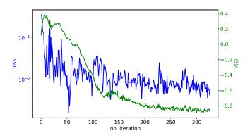
FIG. 14. Online training of NAF agent on LINAC4 trajectory steering in horizontal plane: convergence of loss function and value function V. The latter converges to -0.85 corresponding to an RMS better than 1 mm in case of correction in one iteration.
