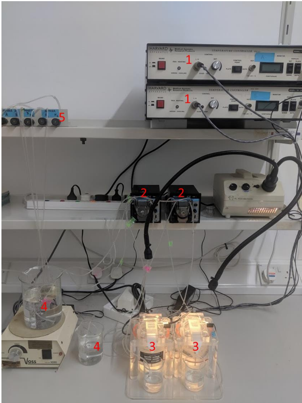
Figure 2.19. General setup of the Hass-type interphase chambers. 1 - TC-202A Bipolar Temperature Controller (Warner Instruments); 2 – Two-channel peristaltic pump; 3 – Haas-type slice chamber; 4 – aCSF (+/-) glucose; 5 – Ggs regulators.
