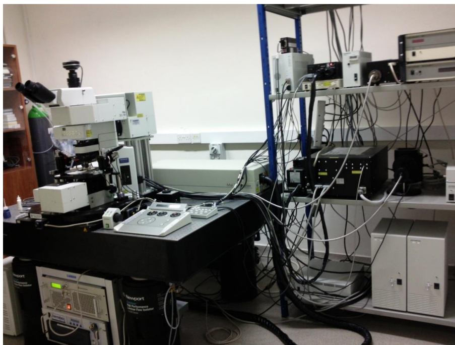
Figure 2.12. FV1000 MPE Olympus Multiphoton microscope (Olympus, Tokyo, Japan).
