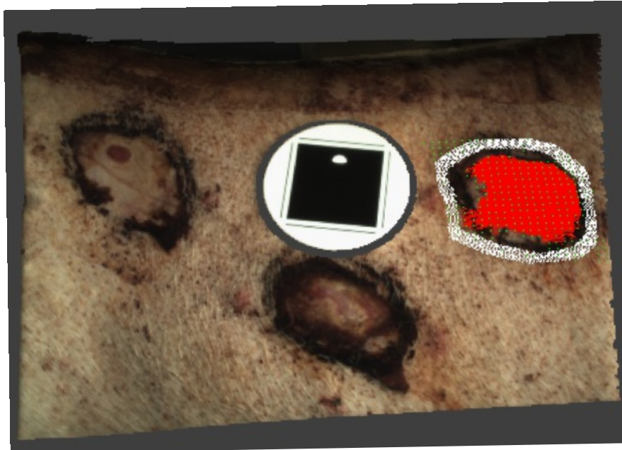
Figure 3.2.30: A photographic image of the wound area measurement on a pig flank using the Eykona camera. The wound area measured in this example is highlighted in red and outlined in white. The central white disc with a black rectangle is the target needed for recognition by the device.
