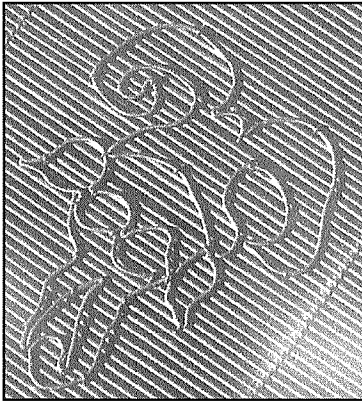
The watermark was a piece of brass which was stitched to the mould.
