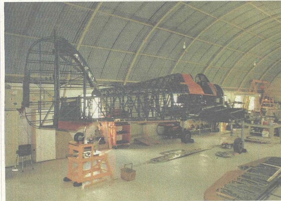
The fuselage of the Hawker Hurricane prior to being covered by fabric.
