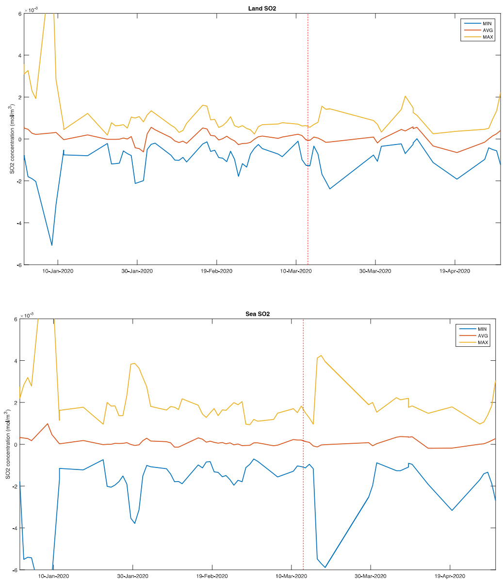
Figure 17. Min, mean, and max SO 2 over land ( top ) and over sea ( bottom ) in the Malta Channel domain.
