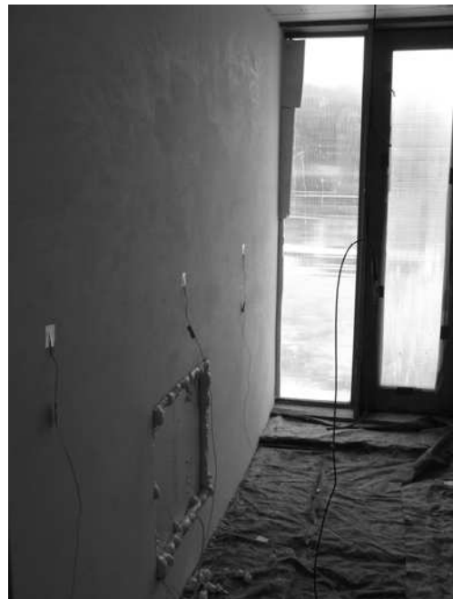
Figure 1. Experimental wall (gypsum-PCM).
