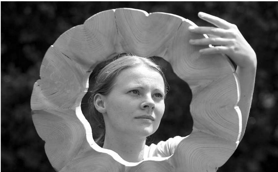
Figure 7. Ring-shaped cross section made of densified half-round timber
