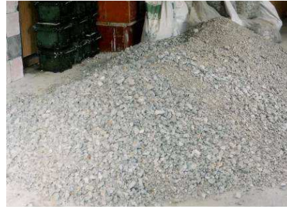
Fig. 4 – Material after secondary crushing
