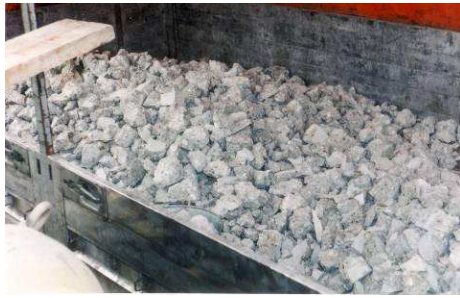
Fig. 3 – Material after primary crushing
