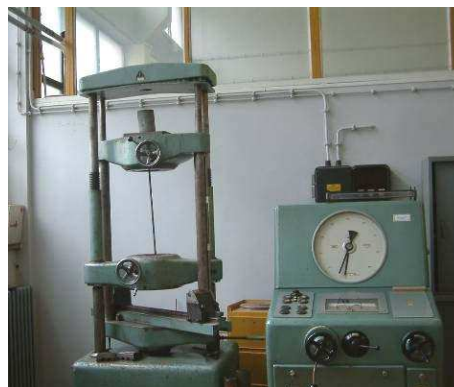
Fig. 7 – Testing of bond between concrete and reinforcement
