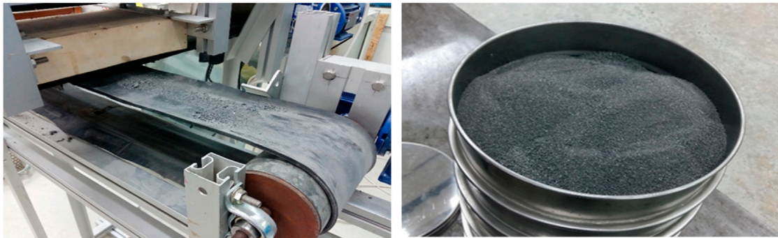
FIGURE 2 | Fiber separator machine at the University of Malta and crushed recycled UHDC.
