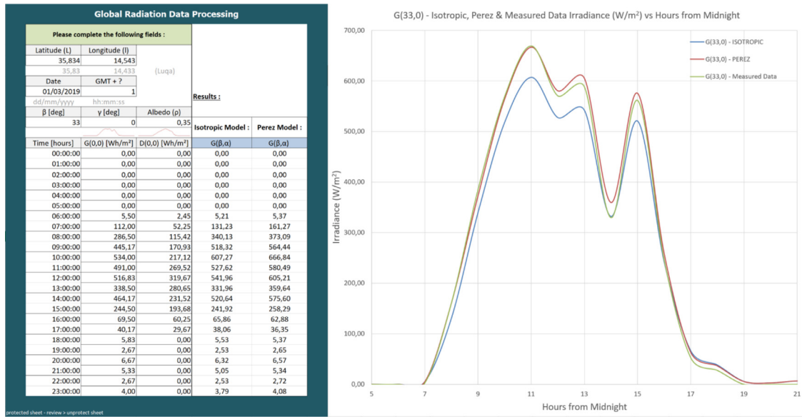
Fig. 5. Comparison file user interface and overcast sky simulation result.
