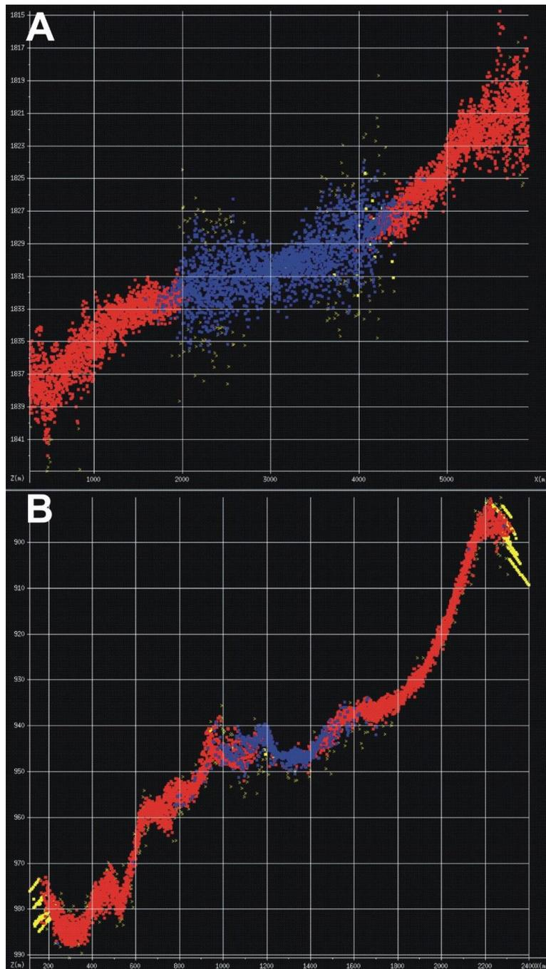
Figure 23: Screenshot of Caraibes editing tool showing increased vertical spreading of the soundings away from the nadir. Blue: soundings determined on phase, Red: soundings determined on amplitude and Yellow: soundings flagged as invalid. Note the difference in scatter between the EM122 (A) and EM710 (B) systems.
