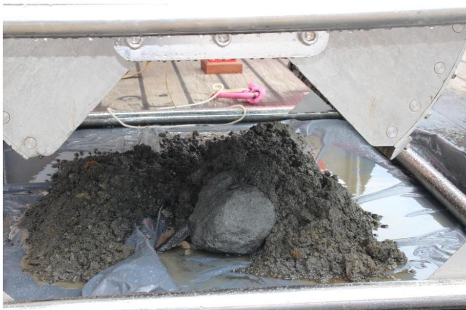
Figure 47: Sample H2, showing the buckets of the HyBIS grab module, and the bulk sample of volcaniclastic gravels with one large, dense rounded block.
