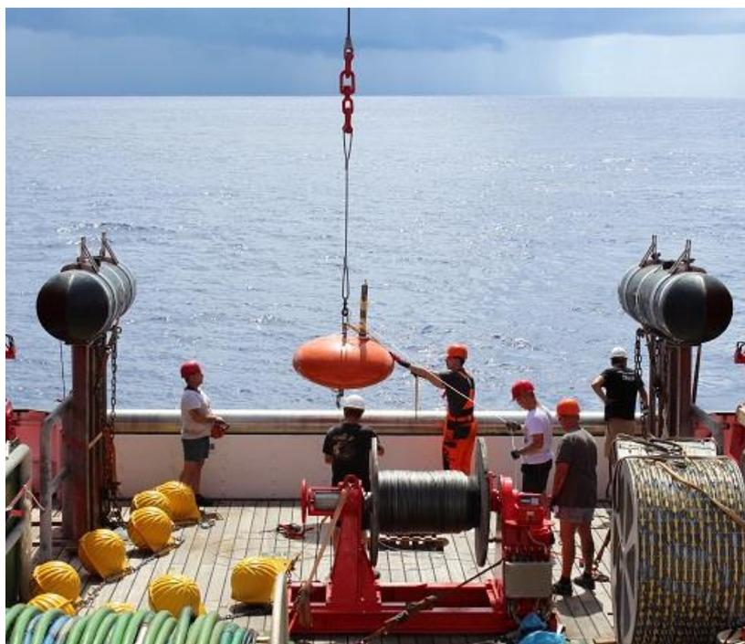
Figure 57: Deployment of the top-buoy of the 7 km long mooring. In the center, the spooling winch with the first 2,000 m of Dyneema rope. To the right, the first drum with 200 m cable holding 100 temperature sensors.
