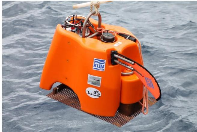
Figure 18: Deployment of the new OBS Nammu from KUM (Photograph: Theresa Roth).
