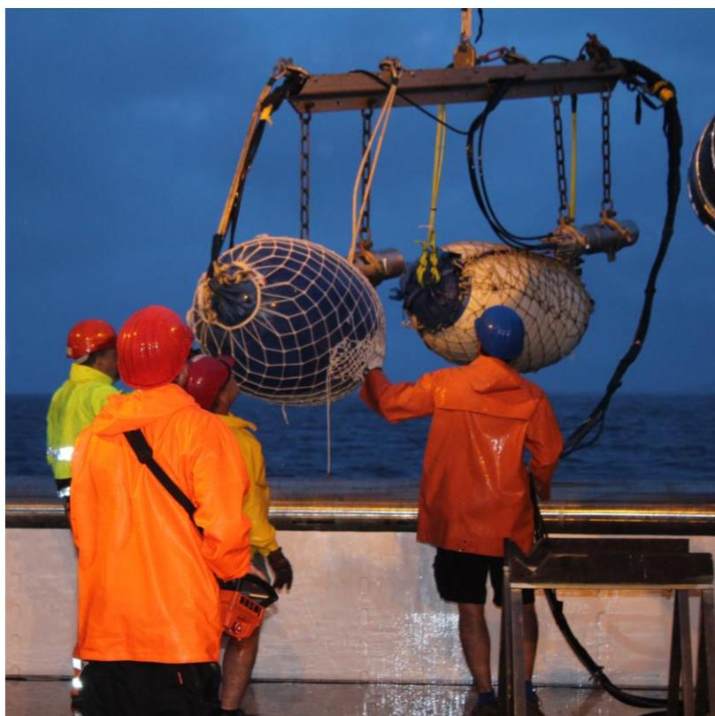
Figure 5: Two standard GI-Guns (105/105 in<sup>3</sup>) were operated in harmonic mode as seismic source during the cruise SO252. (Photographer: Melanie Ray)
