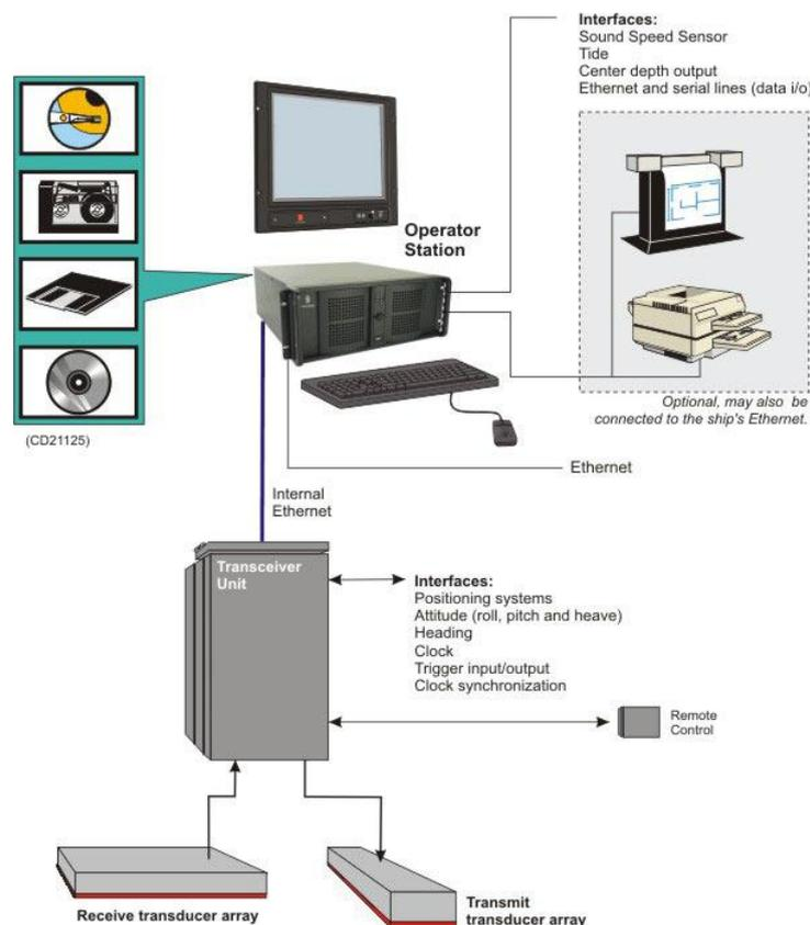
Figure 20: Configuration drawing of the EM122 system units and interfaces.
