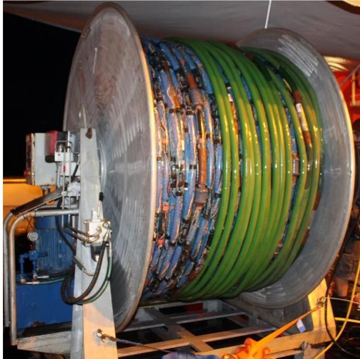
Figure 6: GeoEel streamer segments of 12.5 m length were connected to build up the 2D streamer system. (Photographer: Melanie Ray)
