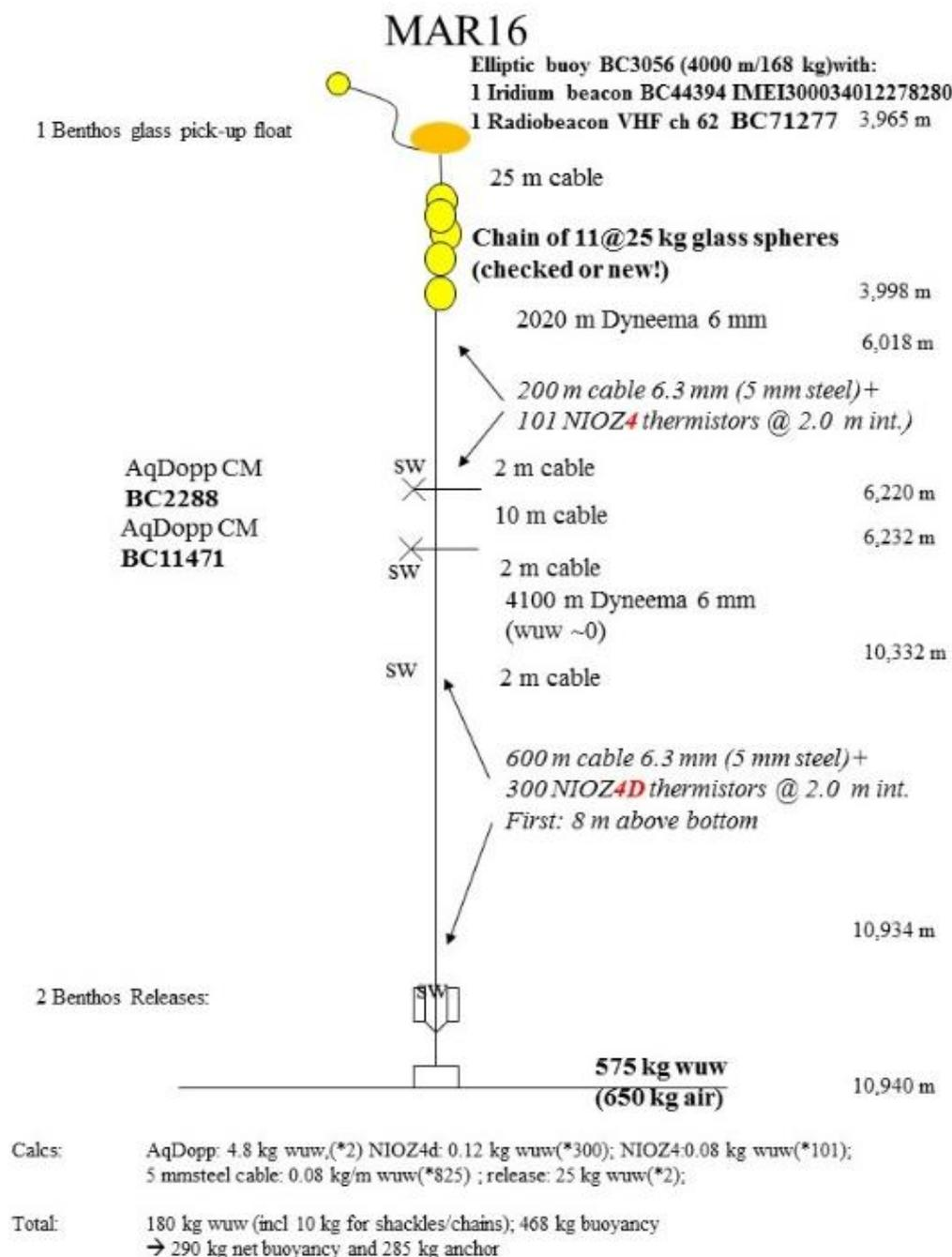
Figure 58: Sketch of the 7 km long mooring with current meters and high-resolution temperature sensors.
