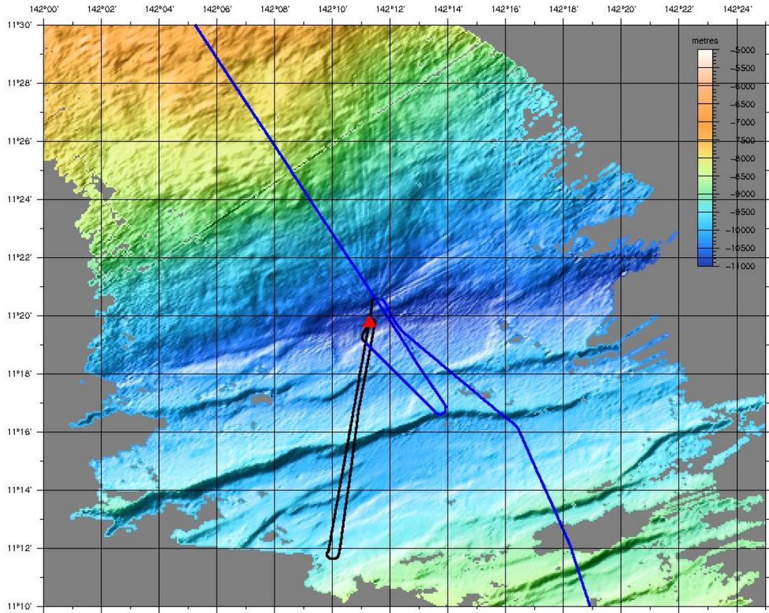
Figure 24: Shaded relief bathymetry of the Marianas Trench. Red star: CTD location. Blue line: High-speed survey ship's track. Black: Low-speed bathymetry survey during mooring lay-out.
