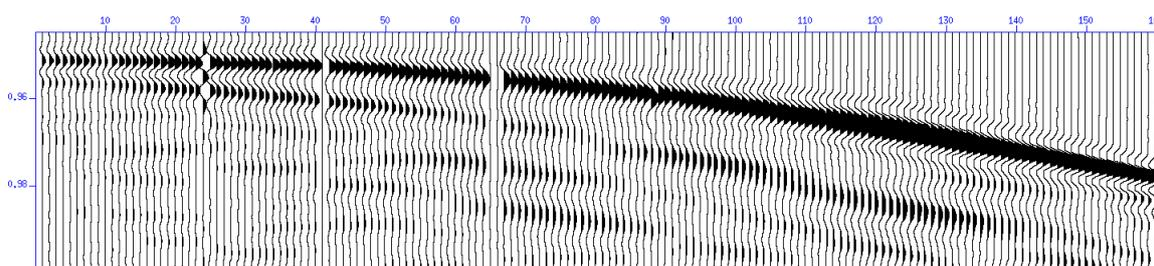
Figure 8: Plotting of the seafloor signal for one shot and 160 channels.
