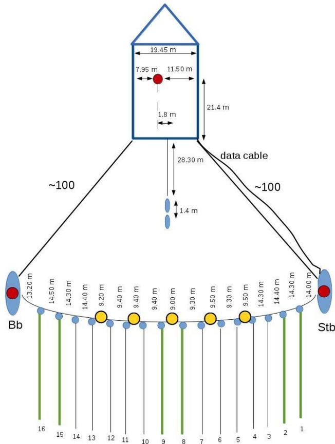
Figure 13: P-cable configuration.
