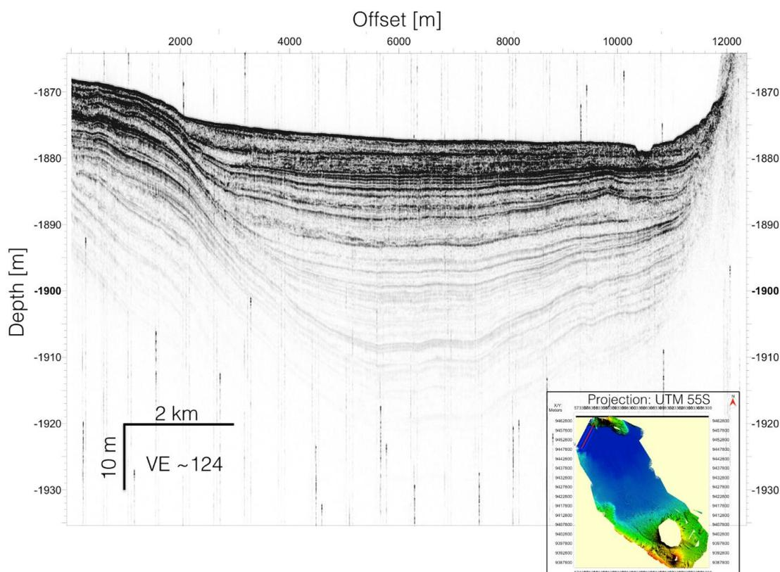
Figure 35: Parasound P70 profile of the secondary low frequency (SLF) of about 4 kHz in the proximal part of Ritter Island inside the Bismarck Sea basin. The x-axis shows offset in m, the y-axis is converted TWT [s] into depth [m] with an average velocity of 1495 m/s derived from the CTD cast. The profile shows high penetration into the seafloor with up to 60 m traceable amplitudes.
