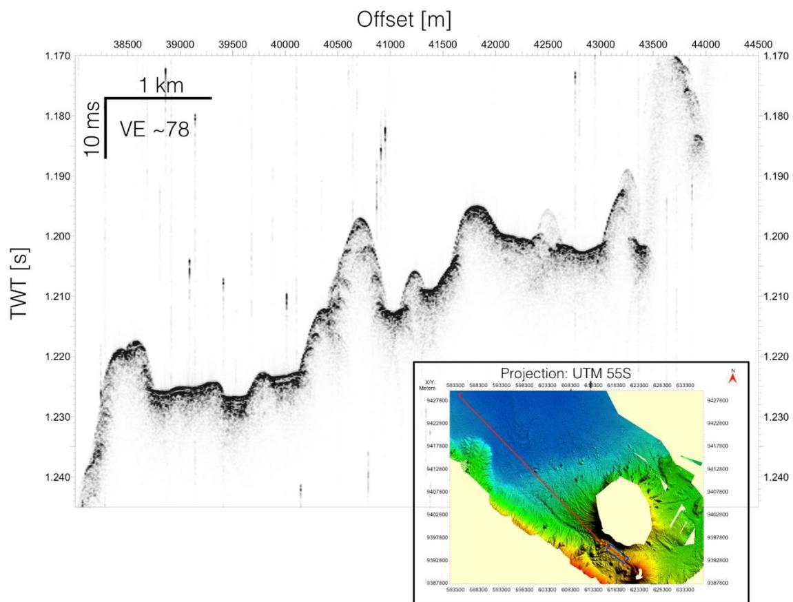
Figure 34: Parasound P70 profile of the secondary low frequency (SLF) of about 4 kHz in the proximal part of Ritter Island in between Sakar Island and Umboi. X-axis is offset in m and y-axis is two-way-traveltime in s. The profile shows low penetration into the seafloor and scattering of energy on mounds and cones.
