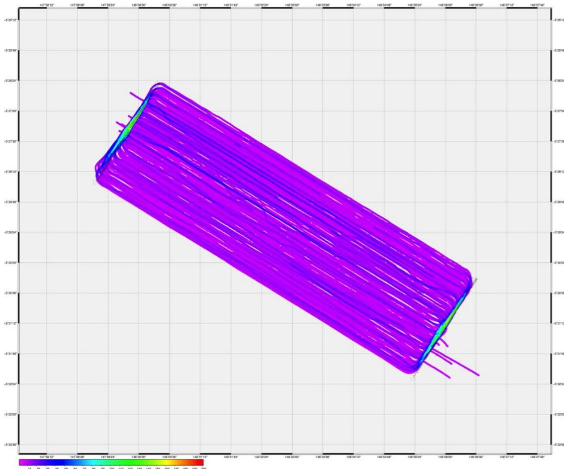
Figure 14: Fold map of the P-Cable survey showing even coverage except for the turns where the ship passed the same location at every sail line.
