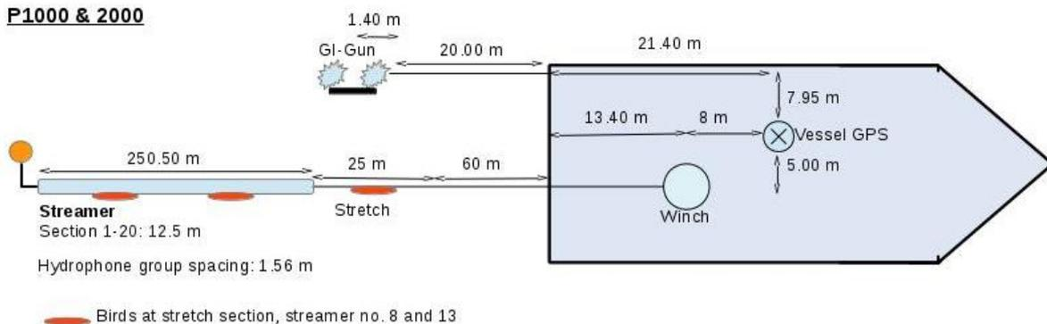
Figure 7: Deck geometries, streamer configuration and gun setting during Cruise SO252.
