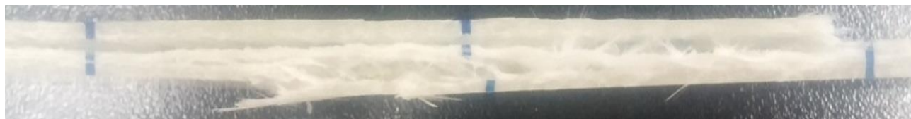
TBI - matrix failure, fibre pull out and delamination
