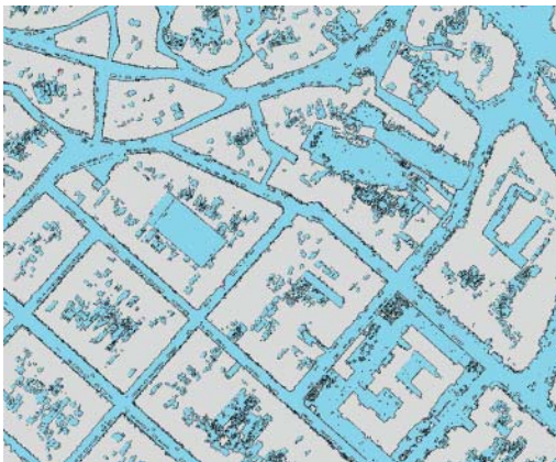
Figure 5: Surface difference between unassigned TIN and all classifications TIN
