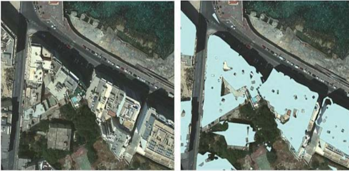
Figure 9: Sliema showing how buildings in close proximity are joined into one polygon
