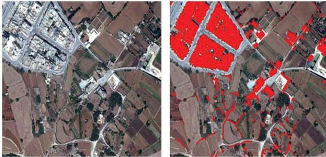
Figure 11: Sliema showing difficulty in extracting building footprint of turf covered roof-top
