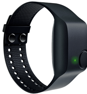
Figure 7.1: The Empatica E4 wristband used for monitoring skin conductance.
