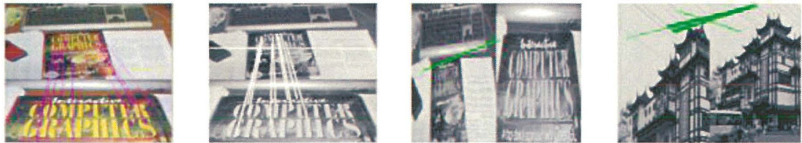
Figure 41: Scale changes comparison. The first result is SIFT (10/66 matches), second is SURF (10/26 matches). The last two images show the results of PCA-SIFT in scale changes. Image from [34].
