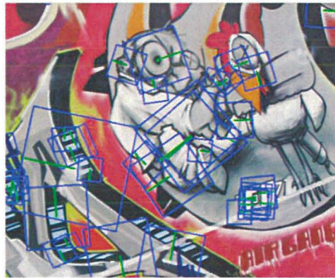
Figure 17: Descriptor Windows - Each window is 20 times the size of the scale of the detected point and is oriented along the dominant direction shown in green. Image from [27].
