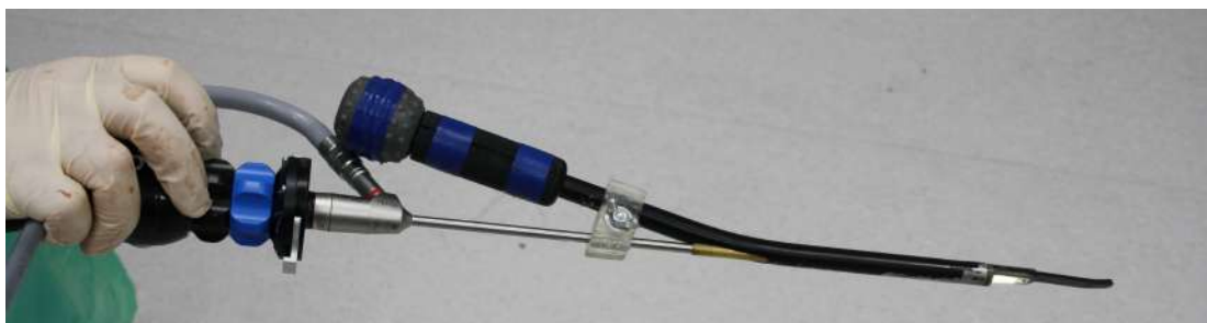
Figure 11: The developed integrated retractor with the 5mm 30-degree endoscope inserted and fixed in place. The tips of the retractor are collapsed. Side view. Additional images can be seen in Appendix 6
