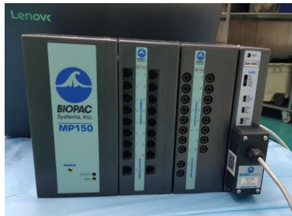
Figure 21b: The receiving unit for the pressure recording system used for these experiments.
