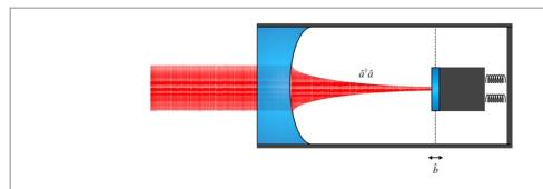
**Figure 1.** An optomechanical system consisting of a moving end mirror. The operators  $\hat{a}$  and  $\hat{a}^{\dagger}$  denote the creation and annihilation operators for the light field, and  $\hat{b}$  and  $\hat{b}^{\dagger}$  denote the motional degree of freedom of the mirror. Other examples of optomechanical systems include levitated nanobeads and cold-atom ensembles.
