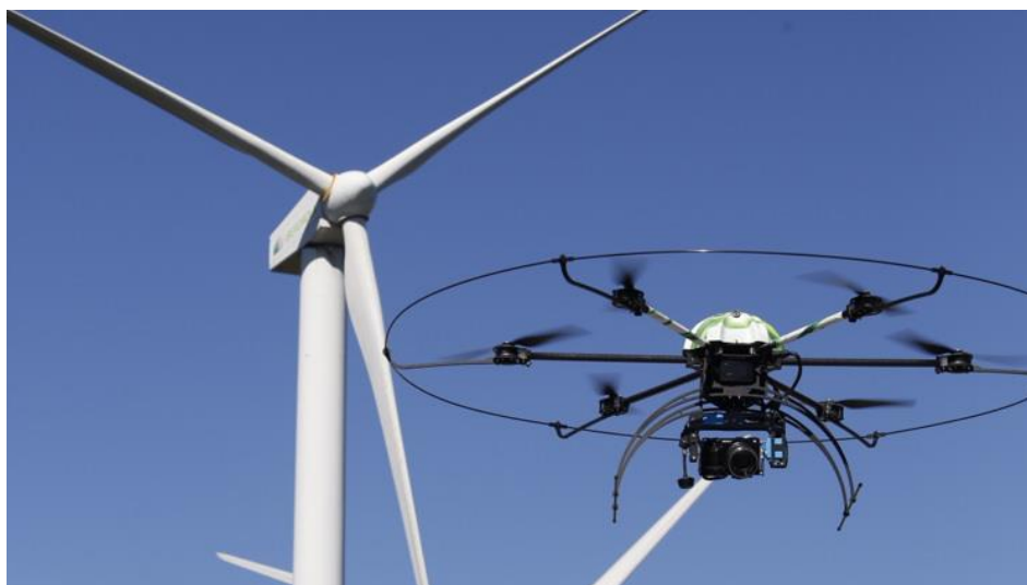
Figure 1.1: The Arachnocopter drone from Iberdrola used for the detection of damage on wind turbine blades [29].
