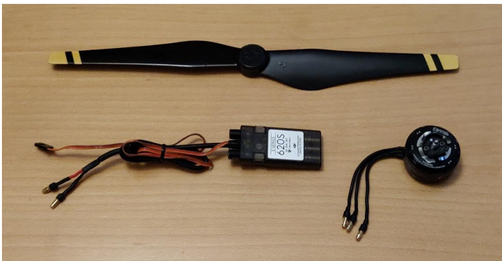
Figure 4.5: DJI 1345 propeller, E-series 620S ESC, and a DJI 3510 brushless DC motor, utilized for the propulsion system of the research UAVs.
