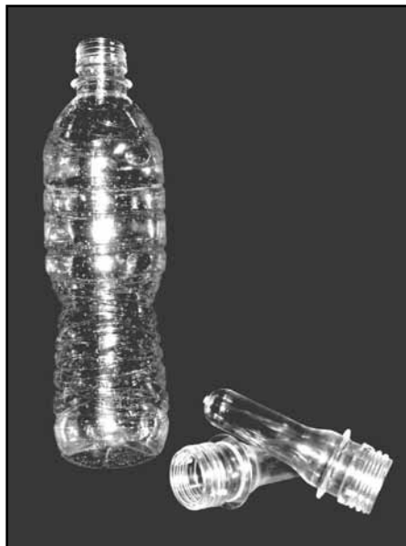
PET bottle preforms before being transformed into a finished plastic bottle by injection blow moulding processes.
