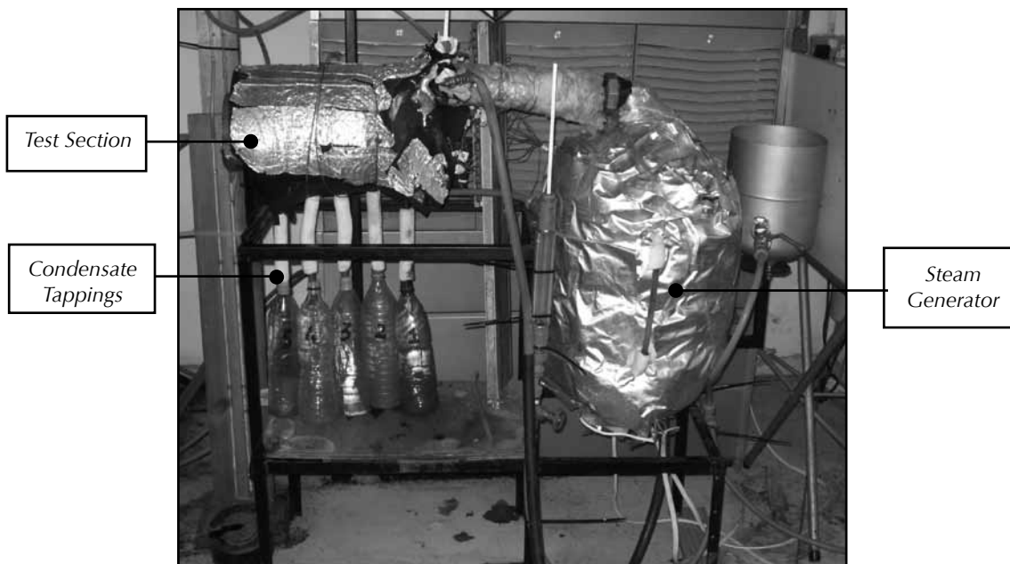
The testing equipment
