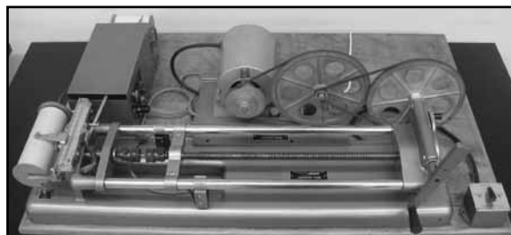
Figure 2: The restored Hounsfield Tensometer
