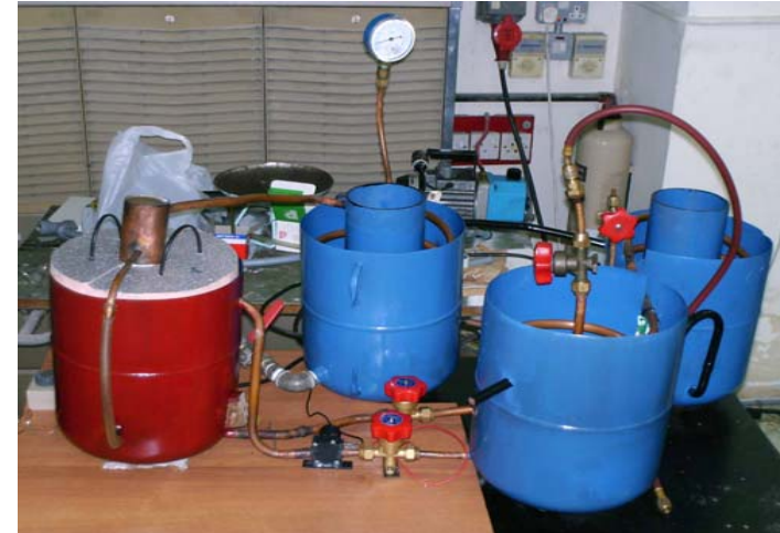
The fully assembled vapour absorption refrigeration test rig
