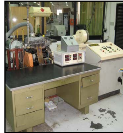
Manual system: Engine, Dynamometer and control console
