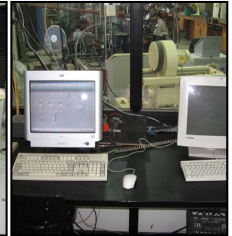
Control Room: Monitor and control engine from PC
