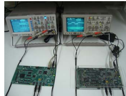
Figure 1 – DSK6416 (right) carrying out FSK modulation and demodulation; DSK6713 (left) generating noise and using the generated noise to corrupt the QAM signal of the DSK6416 prior to demodulation.
