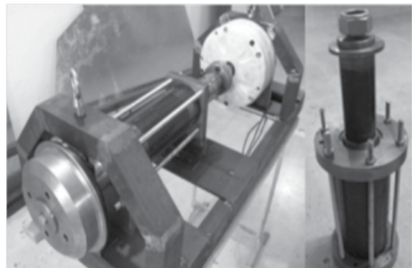
Figure 2: Nacelle and Yaw system
