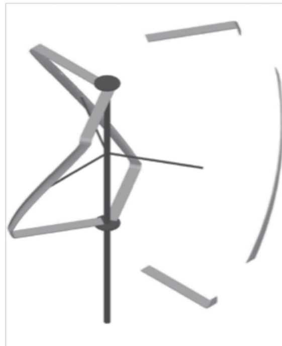
Figure 1 VAWT conceptual design showing an unassembled blade.
