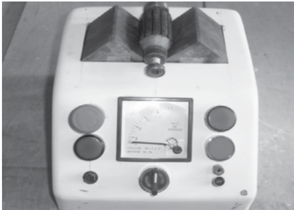
Photo 1: shows the armature growler and insulation tester
