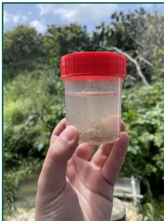
A typical sample collected to quantify suspended sediment concentration.
