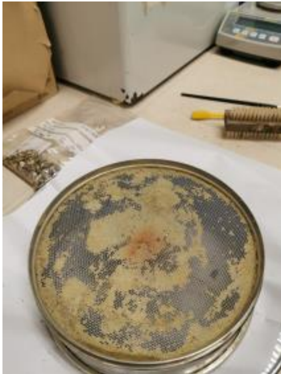
Figure 6: A pre-folded A3 sheet of paper is placed on a tray. The sieve is then placed upside down for the inclusions to fall on the paper.
