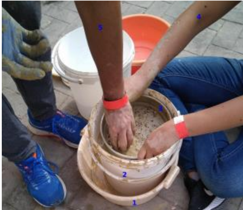
Figure 4: Sieving procedure and equipment. A bucket (2) is placed in a tray (1) whilst the sieve (3) is held on top of the bucket by Person 1 (4). Person 2 (5) is breaking the lumps of clay.
