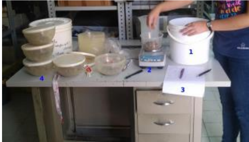
Figure 3: The soaking equipment. 1: initial sample; 2: electronic scale; 3: written record; 4: soaked samples in labelled plastic boxes
