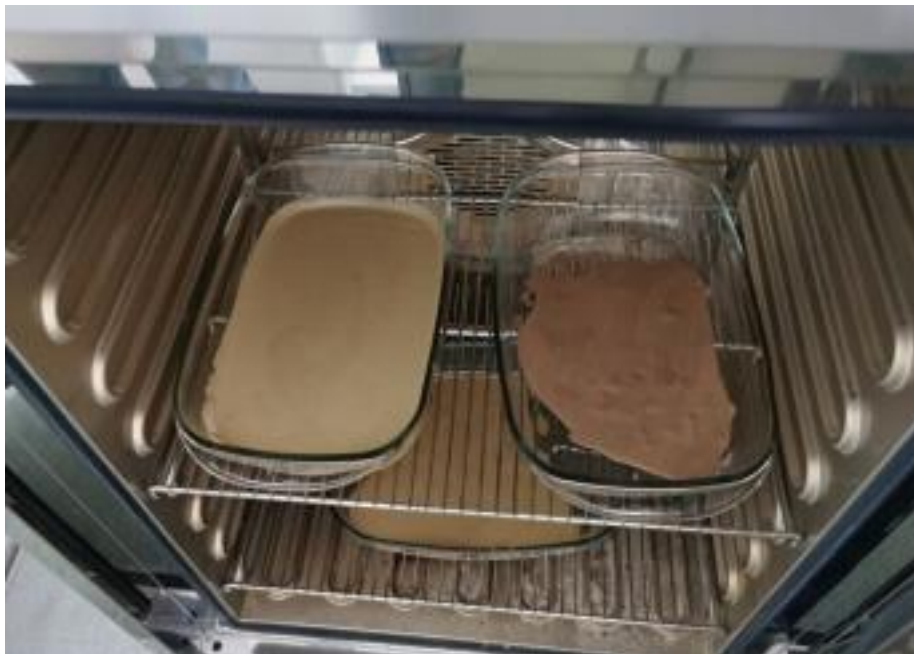
Figure 10: The clay-water mix is poured in glass trays which are placed in the drying oven.
