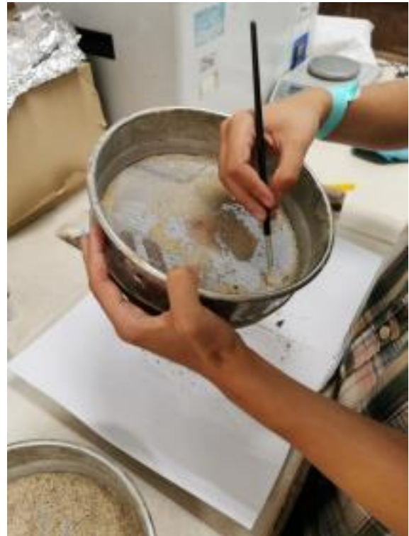
Figure 7: A paint brush can be used to detach the inclusions from the sieve.
