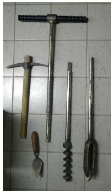
Figure 2: Equipment used during clay sampling. From left to right: pick axe, archaeological trowel, handles with extension rod, spiral auger, auger for stony soil
