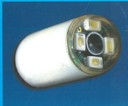
Figure 1: The endoscopy capsule measures 26x11mm.
